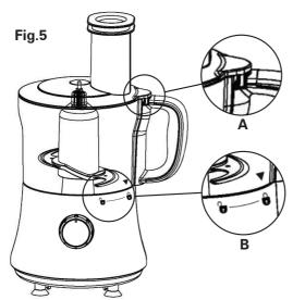
To operate the processor, always ensure the processor lid (Fig.5A) and the processor bowl (Fig.5B) are securely locked into place with the markings lined up.
